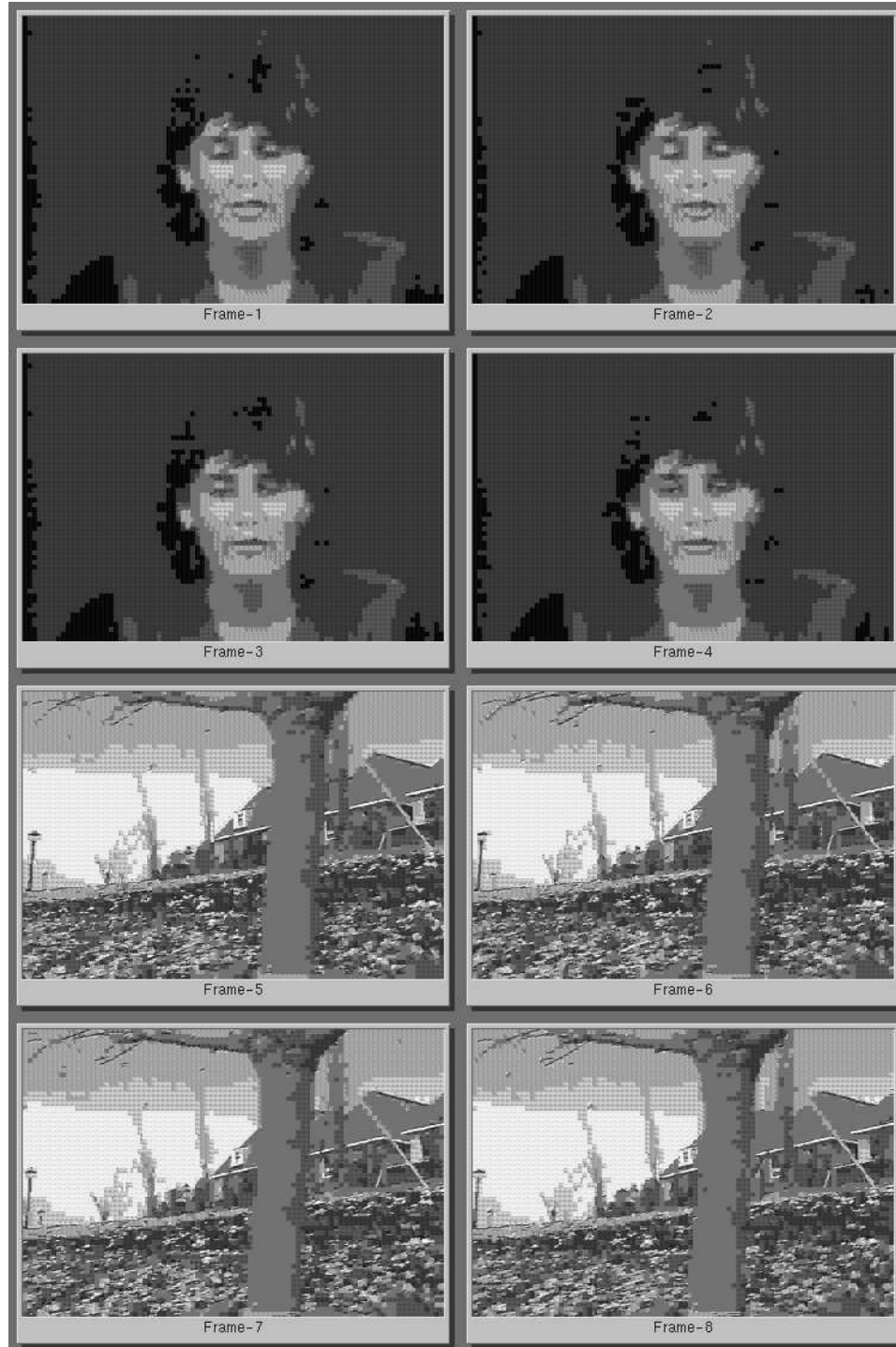
Figure 9.22: Quantized image sequence for the GTR algorithm for 16-dimensional vectors and a local codebook of 256 codewords ( \lambda = 209 , \text{MSE} = 379.5 , \text{rate} = 0.271 bits/pixel).
