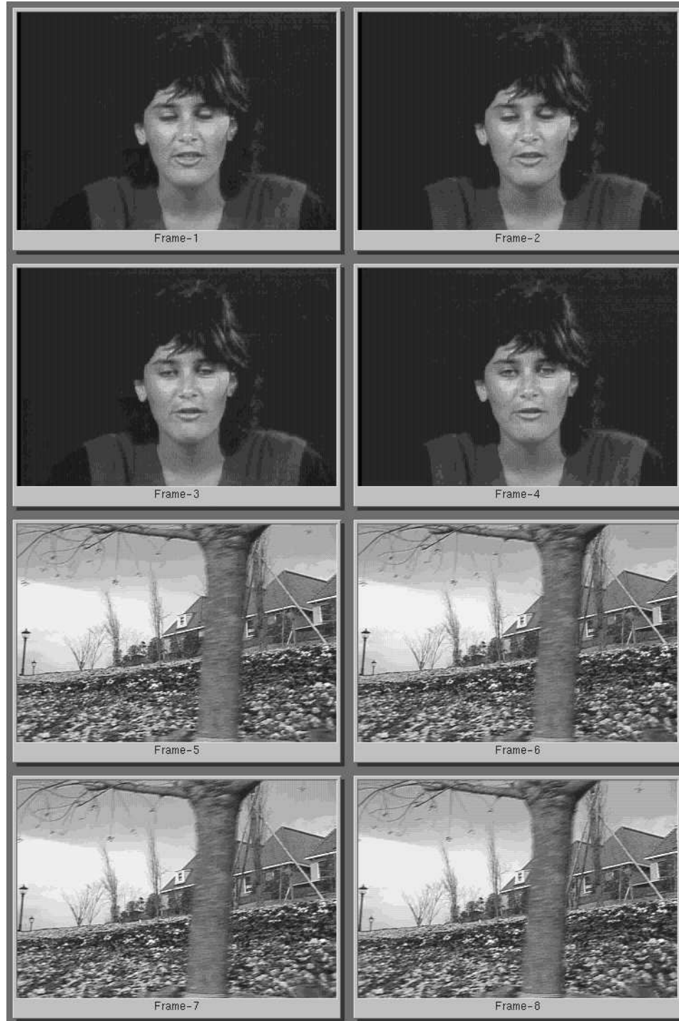
Figure 9.18: Quantized image sequence for the GTR algorithm for 4-dimensional vectors and a local codebook of 256 codewords ( \lambda = 16 , MSE = 38.6 , rate = 1.522 bits/pixel).
