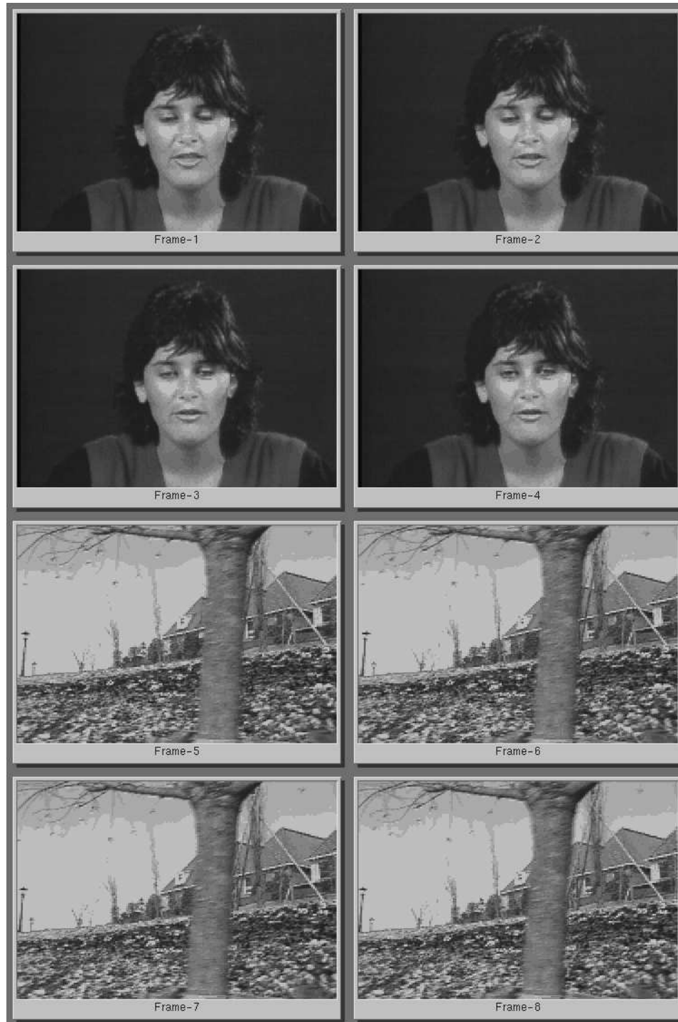
Figure 9.19: Quantized image sequence for nonadaptive VQ for 4-dimensional vectors and a VQ codebook of 256 codewords (MSE = 234.9, rate = 1.487 bits/pixel).
