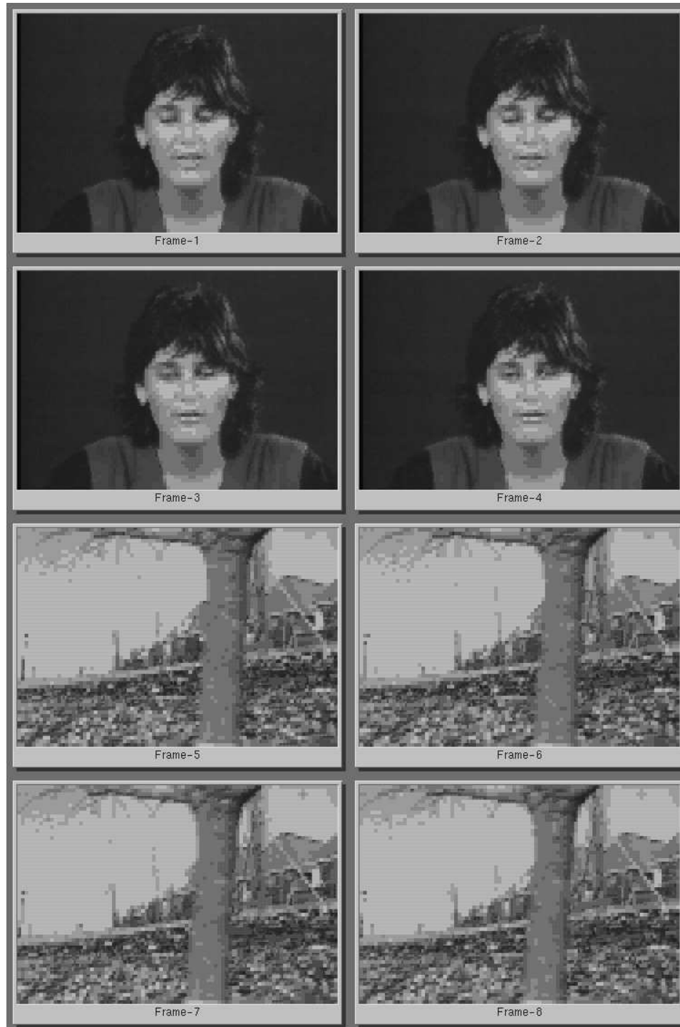
Figure 9.23: Quantized image sequence for nonadaptive VQ for 16-dimensional vectors and a VQ codebook of 256 codewords ( MSE = 502.1 , rate = 0.322 bits/pixel).
