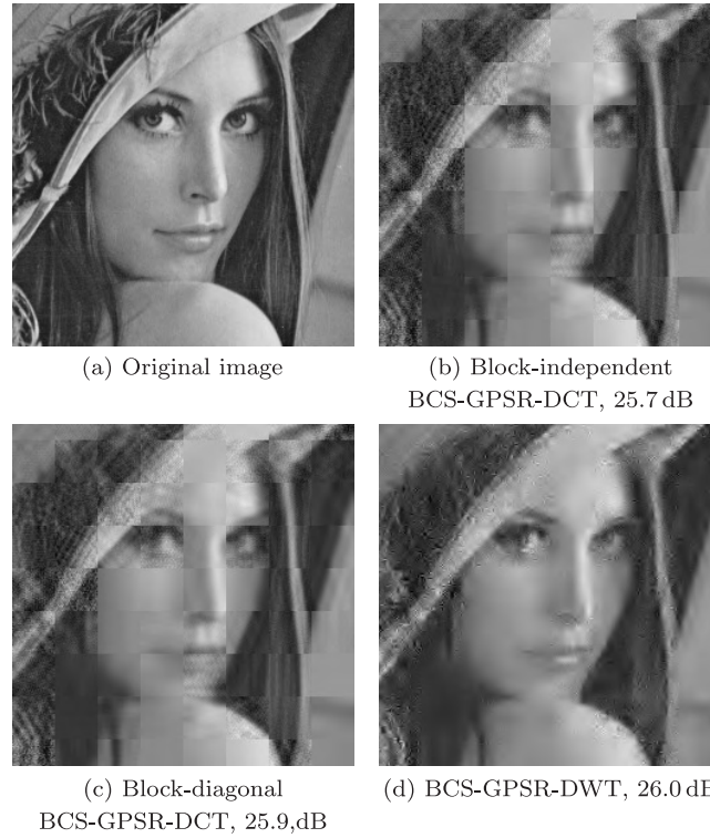
Fig. 3.3 Reconstructions of the 512 \times 512 “Lenna” image (shown in detail) for a subrate of S = 0.2 . BCS measurement uses 32 \times 32 blocks.
