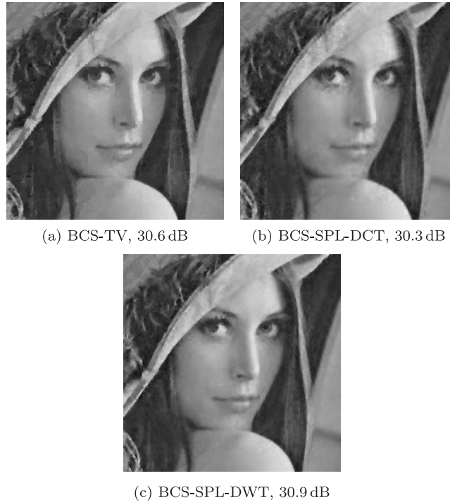
Fig. 3.4 Reconstructions of the 512 \times 512 “Lenna” image (shown in detail) for a subrate of S = 0.2 . BCS measurement uses 32 \times 32 blocks.
